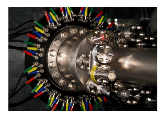
A probe for the magnetic order: The Swiss muon source at the Paul Scherrer Institute enables the researchers to observe the anti-ferromagnetic order in very thin films. The sample is introduced via the main access to the measuring chamber. The colourful contacts are used to connect the positron detectors. © LMU/Paul scherrer Institute
