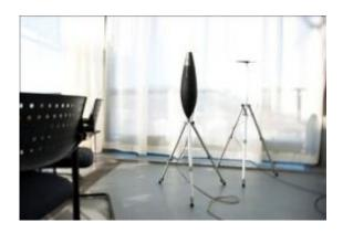
Acoustic tests with the new sound-absorbing curtain in a normal living room: measuring the reverberation time with a loudspeaker and microphone.
