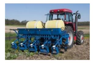
The multipurpose cover crop seeder prototype, designed and built by Penn State agricultural scientists, could save farmers \$10 to \$20 an acre by performing two to three operations at once. The seeder scores the soil, plants seed, adds herbicides and sprays fertilizer in a single trip. Credit: Patrick Mansell, Penn State
