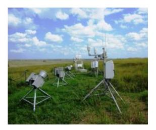
Spectral radiometers measuring sunlight wavelengths in the sky over Oklahoma at DOE's ARM Climate Research facility.
