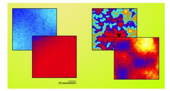
Results of measuring graphene on a boron nitride substrate are at left, graphene on silicon dioxide at right. The STM mapped both the topography of the systems (back) and the local charge densities (front). Graphene on boron nitride is extraordinarily flat, and inhomogeniety of local charge states is signicantly reduced compared to silicon dioxide.
