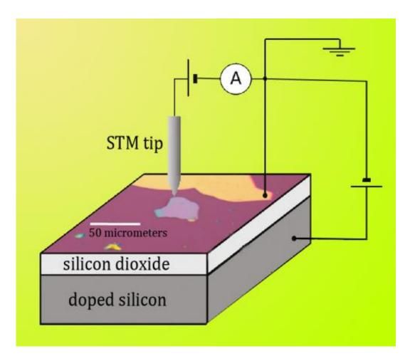
The researchers deposited boron nitride flakes on a layer of silicon dioxide, grown on a layer of doped silicon. The doped silicon was used as a gate electrode for doping the graphene during scanning tunneling microscopy. Graphene was applied to both the boron nitride flakes (under the STM tip) and the bare silicon dioxide; the graphene (dark and light purple) was grounded by an electrode of gold/titanium (gold). The STM could scan across both substrate systems.
