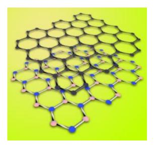
Graphene (top layer) is a hexagonal arrangement of carbon atoms. Hexagonal boron nitride is a similar arrangement of boron and nitrogen atoms whose lattice constant is just 1.7 percent larger. Boron nitride's attributes make it an excellent substrate for preserving graphene's intrinsic properties.
