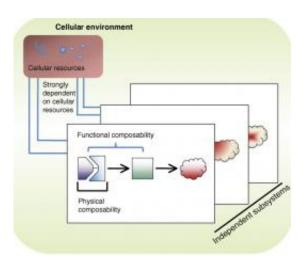
Synthetic biologists want to design biological circuits from scalable families of interconnecting parts. Multiple independent biological circuits (subsystems) composed of interconnected parts (lines) would share the same resources inside a single cellular environment. Credit: Courtesy of Adam Arkin group
