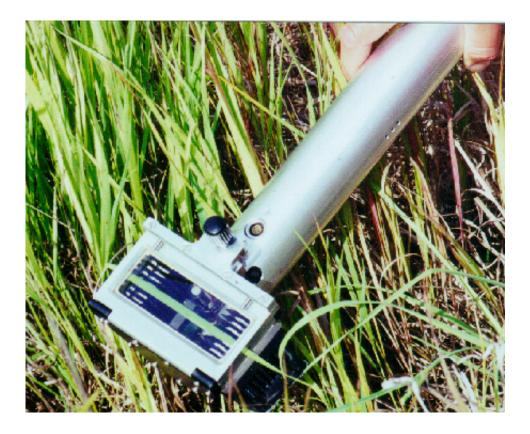
The portable carbon dioxide gas exchange system measures grass leaf photosynthesis. Credit: BioCON Experiment/NSF Cedar Creek LTER Site
