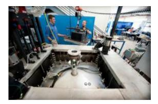
NREL researchers Dirk Long, left, and John Ireland attach the cover on the calorimeter that the group designed and built to conduct advanced research on batteries at the Thermal Test Facility at NREL. Credit: Dennis Schroeder
