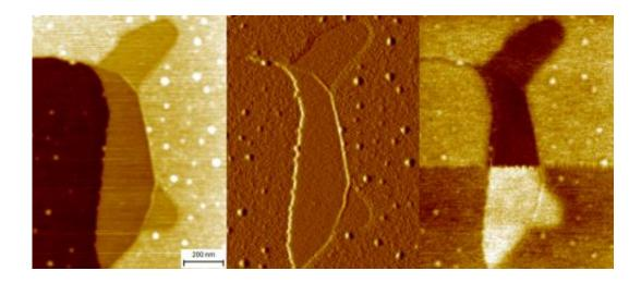
The left hand image is the topography; the middle the topography error image; and right the electrostatic force microscopy image where the tip bias has been switched half way through the image.
