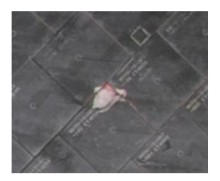
This undated image made available by NASA on Friday, May 20, 2011 shows a damaged thermal tile on the space shuttle Endeavour's underbelly. The crew is planning to use a laser-tipped boom early Saturday, May 21, 2011 to inspect the gouge which is about the size of a deck of cards. (AP Photo/NASA)
