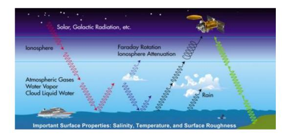
Many natural sources, besides salinity, contribute to the microwave radiation at L-band frequencies (approximately 1 gigahertz) measured by satellites. Correcting the influence of these natural sources is a key to obtaining Aquarius' accurate salinity measurements. Image credit: NASA
