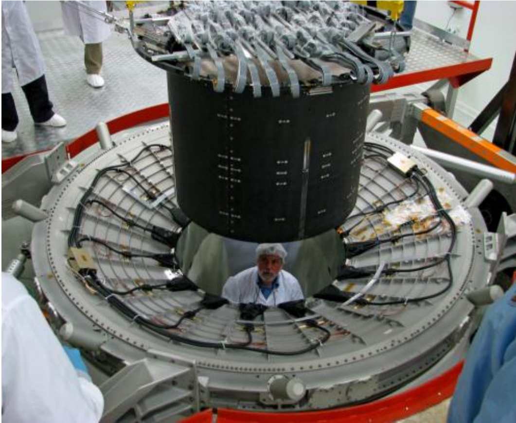
Assembling the AMS-02 magnet. Credits: CERN / AMS-02 Collaboration
