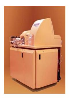
The CyTOF instrument used to carry out mass cytometry. The apparatus can measure the physical traits of as many as 1,000 single biological cells per second. Credit: Image credit: Sergey Vorobiev, DVS Sciences Inc.
