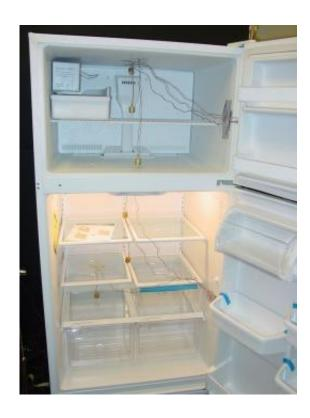
One of four types tested by NIST researchers, this top-mount refrigerator freezer was outfitted with three thermocouples in each compartment, sampling the temperature every 30 seconds. In all units tested, electric heaters used to free ice from molds accounted for about three-quarters of ice-maker energy consumption. Credit: NIST
