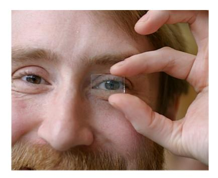
Richard Lunt, one of the researchers who developed the new transparent solar cell, demonstrates its transparency using a prototype cell. Photo: Geoffrey Supran
