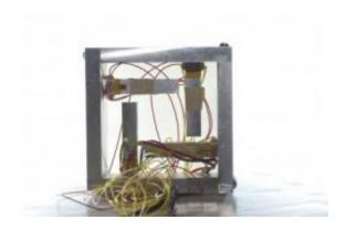
Custom sensors built by Rice engineering students are part of the active handrails that provide force feedback on how heavily patients are depending on their arms as they perform balancing tasks on the Wii boards. Credit: Jeff Fitlow/Rice University
