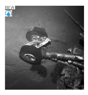
Landing gear from Air France Flight 447 photographed from a REMUS 6000 autonomous underwater vehicle (AUV). (BEA/Woods Hole Oceanographic Institution)
