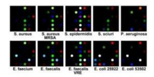
An array developed by University of Illinois researchers demonstrated on 10 common infectious bacteria. The color changes of the sensor array show what kind of bacteria is growing and even if they are antibiotic resistant. Credit: K. S. Suslick
