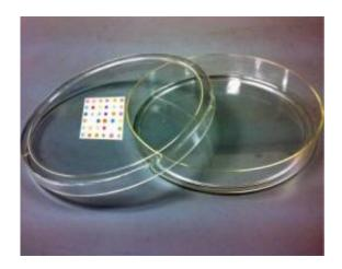
A colorimetric sensor array is placed in an Petri dish for culturing bacteria and scanned with an ordinary flatbed photo scanner kept inside a lab incubator. The dots change color as they react with gases the bacteria produce, identifying specific strains through their aromatic "fingerprints." Credit: K. S. Suslick
