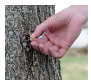
S&T graduate student Matt Limmer uses the SPME, or solid-phase microextraction fiber, to extract a sample from a tree in Schuman Park.
