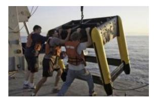
Crew members work with the Triaxus that can conduct rapid 3-D surveys of ocean fronts while towed behind a ship. Credit: UW Applied Physics Laboratory
