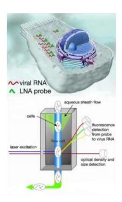
Top: An LNA probe binds to complementary viral RNA inside an infected cell. Thousands of these cells are then run through a flow cytometer (bottom). As the cells pass through a laser, they are excited and the probe fluorescence is measured. Credit: Chemistry Pictures (2006), Union Biometrica (2010)
