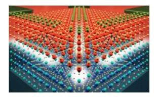
An atomic-scale depiction of the SketchSET shows three wires (green bars) converging on the central island (center green area), which can house up to two electrons. Electrons tunnel from one wire to another through the island. Conditions on the third wire can result in distinct conductive properties. Credit: U. Pittsburgh
