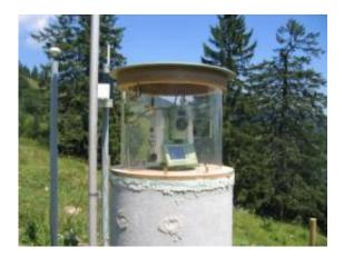
Video-tachometer with laser scanner and camera can detect movements of natural target objects, such as stones or tree stumps. Credit: alpEWAS research group
