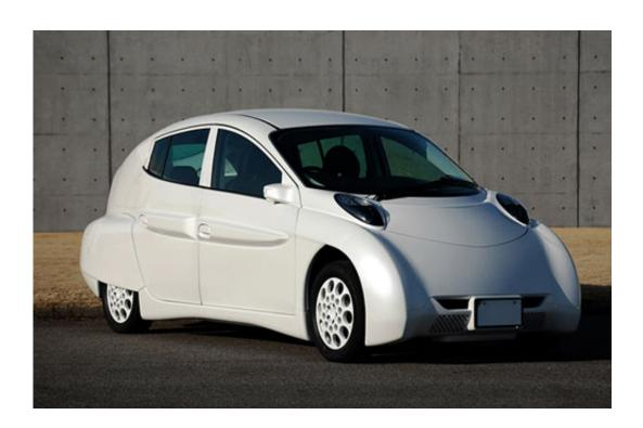
(PhysOrg.com) -- SIM-Drive Corporation, a Japanese consortium based in Kawasaki-shi and comprised of 34 companies and municipalities, has announced that it has developed a functioning electric car based on inwheel electric motor technology.
