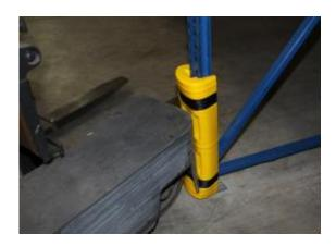
If a forklift collides with the air cushion, a sensor within the protective device sends pressure change information to a central control station. Credit: Fraunhofer IMS
