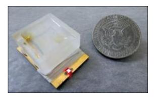
The sensor is self-powered, easy to use, and signals the presence of trypsin via a light-emitting diode (LED) that is visible to the unaided eye. Credit: Brian Zaccheo
