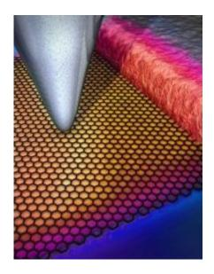
An atomic force microscope tip scans the surface of a graphene-metal contact to measure temperature with spatial resolution of about 10 nm and temperature resolution of about 250 mK. Color represents temperature data. Credit: Alex Jerez, Beckman Institute for Advanced Science and Technology
