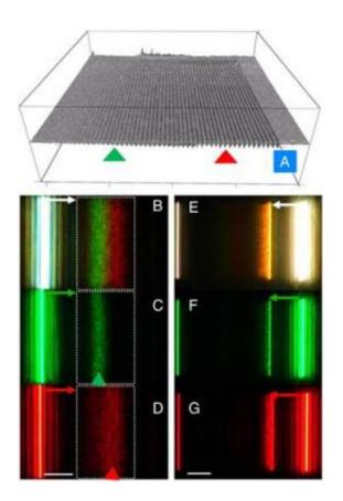
An image of a graded grating obtained with atomic force microscopy. The groove depth (a) increases from approximately 6nm to 100nm. Images b, c and d show emission from the structure with different filters. Images e, f and g are emission images with the SPP modes coupled and propagating in a direction opposite to that for images b, c and d.
