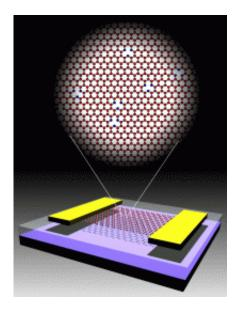
Schematic of a graphene transistor showing graphene (red), gold electrodes (yellow), silicon dioxide (clear) and silicon substrate (black). Inset shows the graphene lattice with vacancy defects. Vacancies (missing atoms) are shown surrounded by blue carbon atoms.
