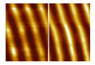
Atomic force microscope image measurements of the same structure in conventional shear mode (left) and using the second resonance regime (right)
