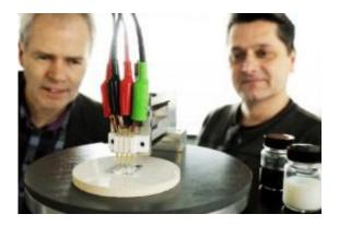
4-point conductivity measurement of the new transparent conducting film developed by Professors Cor Koning (left) and Paul van der Schoot (right). The black pot contains a dispersion of carbon nanotubes in water, and the white pot contains the conducting latex. Credit: Photo: Bart van Overbeeke.
