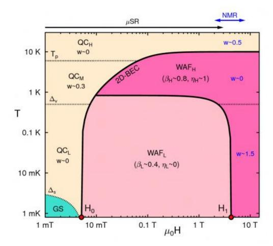
The magnetic field - temperature phase diagram for k-(BEDT-TTF)2Cu2(CN)3 obtained from muon spin rotation experiments and including previously reported NMR and thermodynamic measurements (Credit: Francis Pratt / ISIS / STFC)
