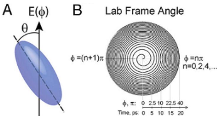
Behavior of molecules in rotationally accelerating strong optical fields. (A) Molecules with nonuniform polarizability tend to align with the electric field vector. (B) Trajectory of the lab frame angle for the electric field during the optical centrifuge pulse, showing the angular acceleration of the field.
