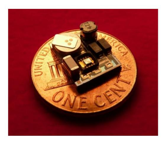
A new energy harvester developed by University of Michigan researchers can harness energy from vibrations and convert it to electricity with five to ten times greater efficiency and power than other devices in its class. Credit: Erkan Aktakka
