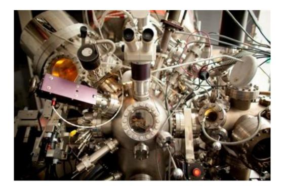
Lehigh's powerful high-resolution X-ray photoelectron spectrometers (HR-XPS), the only of its kind in the U.S., can determine the chemical nature of atoms in a material's surface region and is a perfect complement to the new HS-LEIS. Photo by Douglas Benedict
