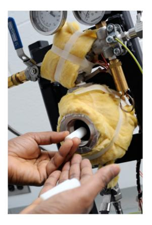
The supercritical aerogel dryer was built by UA polymer engineering graduate student Andrew Shinko.
