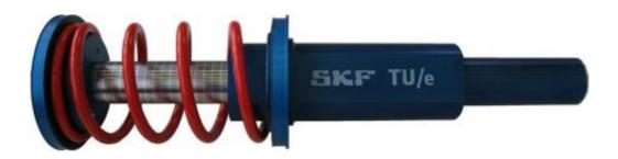
The electromagnetic suspension prototype developed by Eindhoven University for SKF
