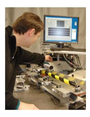
A laboratory prototype of Oak Ridge National Laboratory's Reticle Compensating Rifle Barrel Reference Sensor allows Slobodan Rajic to fine-tune the technology. The system precisely measures the deflection of the barrel relative to the sight and then electronically makes corrections. Credit: Ron Walli
