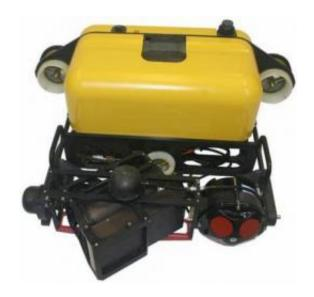
The Explosive Ordnance Disposal Hull Unmanned Underwater Vehicle Localization System can maneuver under ships to detect explosives. Funded by the Office of Naval Research, is closer to reality following the awarding of a production contract in March. Credit: Courtesy photo
