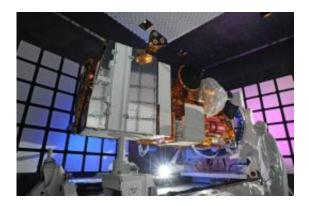
A photograph shows NPP undergoing electromagnetic interference testing. Credit: Ball Aerospace
