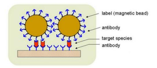
This diagram illustrates how a new sensor technology developed at Oregon State University might work using magnetic beads. (Graphic courtesy of Oregon State University)
