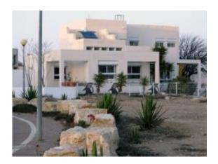
The south-facing windows of a Neve Zin home are designed to capture the low winter sun for passive heating, but can be shuttered to block the higher summer sun to prevent overheating. Credit: ISNS | Alan S. Brown
