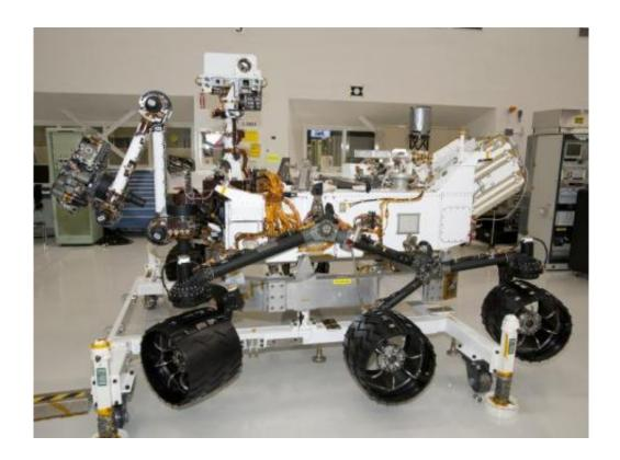
The rover for NASA's Mars Science Laboratory mission, named Curiosity, is about 3 meters (10 feet) long, not counting the additional length that the rover's arm can be extended forward. The front of the rover is on the left in this side view. Credit: NASA/JPL-Caltech
