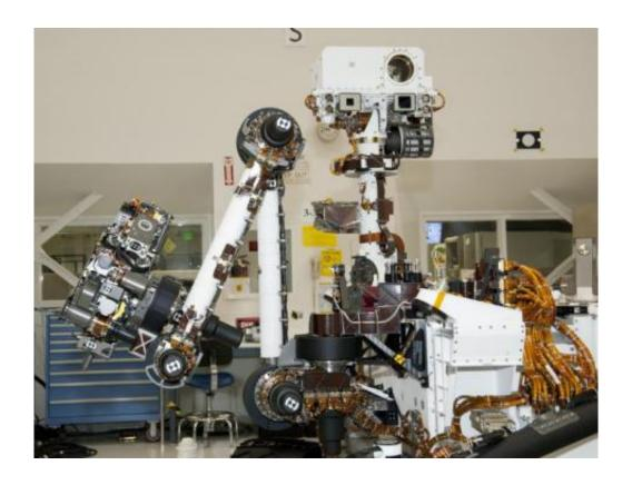
Curiosity's arm and remote sensing mast carry science instruments and other tools for the mission. This image, taken April 4, 2011, inside the Spacecraft Assembly Facility at JPL shows the arm on the left and the mast just right of center. Credit: NASA/JPL-Caltech
