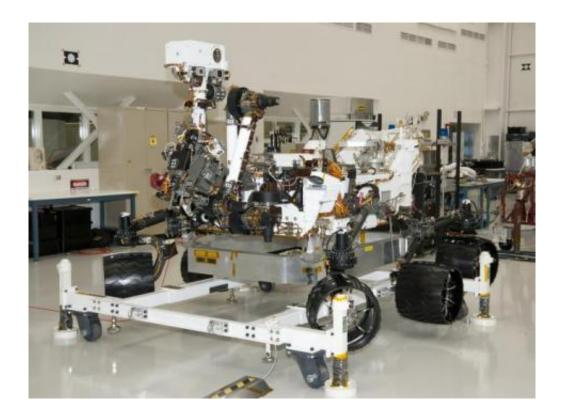
Support equipment is holding the Mars rover Curiosity slightly off the floor. When the wheels are on the ground, the top of the rover's mast is about 2.2 meters (7 feet) above ground level. Credit: NASA/JPL-Caltech
