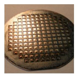
A fully functional solid-oxide fuel cell membrane wafer. The structured surface of each square chip lends stability to the incredibly thin film that is used for the electrochemical membrane. Credit: Shriram Ramanathan.
