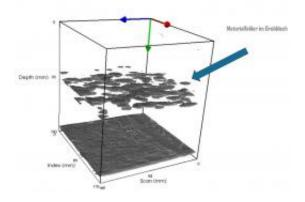
Thanks to a new ultrasound method, material defects can now be displayed in three dimensions. (© Fraunhofer IZFP)
