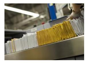
Letters in up to B5 format are separated at high speed at the feeder of the mail sorting machine. Further processing is carried out at a transport speed of four meters per second.
