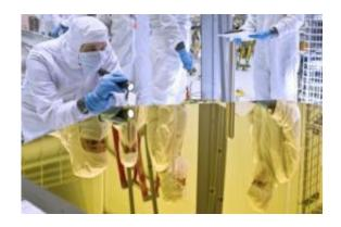
An engineer examines the Webb telescope primary mirror Engineering Design Unit segment in the clean room at NASA's Goddard Space Flight Center, Greenbelt, Md. Credit: NASA/Chris Gunn
