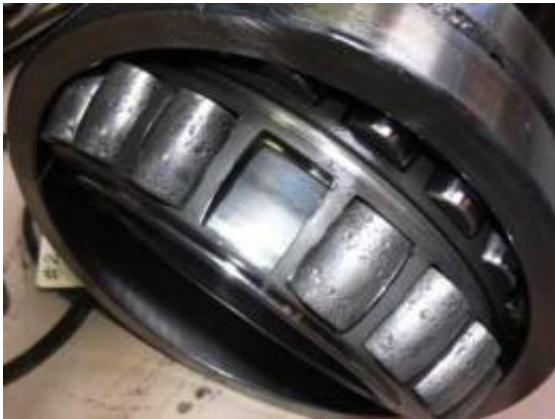
A damaged bearing from a wind turbine gearbox. Photo courtesy NREL.
