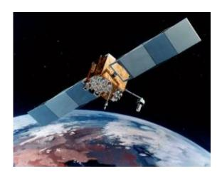
Navstar-2F satellite of the Global Positioning System (GPS). Image: USAF
