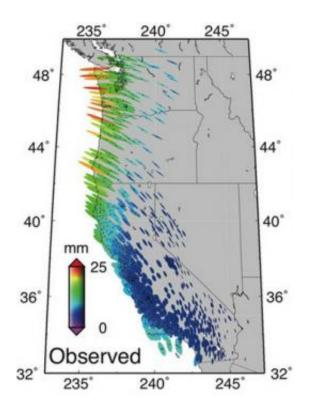
The outline of each ellipse represents the motion the ground makes as the earth flexes in response to the time and space dependent ocean tides. There is an ellipse for each of the GPS sites used in the study, and the color indicates the amplitude of the tidal response movement.
